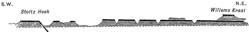
FIG. 60.—Section west of Beaufort West, showing intrusive diabase in the Beaufort Series. After E. H. L. Schwarz. The diabase is shown by the black line.
