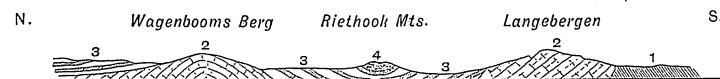
FIG. 11.—Section from the Langebergen to Wagenbooms Berg: 4. Witteberg Series; 3. Bokkeveld Series; 2. Table Mountain Series; 1. Malmesbury Series. Scale: 1 inch=3 miles. (From Cape Geol. Survey Rep. 1897.)
